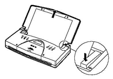
☐ If the leading edge of the jammed sheet is coming out of the paper exit slot, pull the paper out carefully from the paper exit slot.
